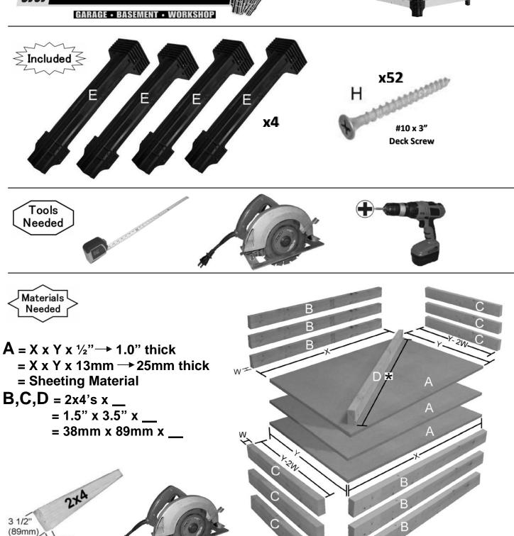
\* This diagonally placed 2x4 helps support the worktop. It is best cut to fit, but the length can be calculated as:
